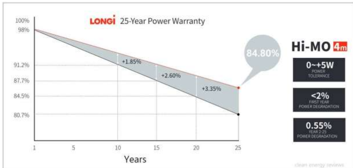
Figure 4: Solar panel performance warranty chart showing degradation over 25 years of use
