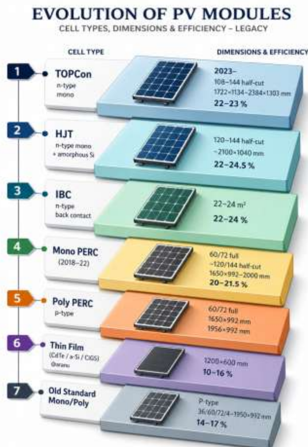
Figure 2: Evolution of solar PV modules: dimension and efficiency legacy
