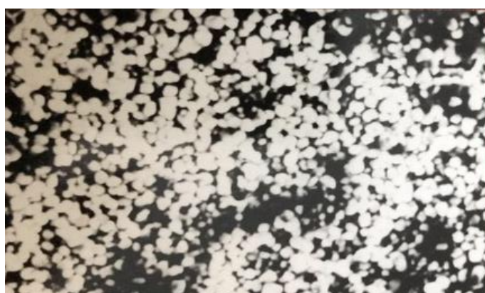
Fig.3. Microstructure of the TiC-TiN-Al 2 O 3 system, X1500.
