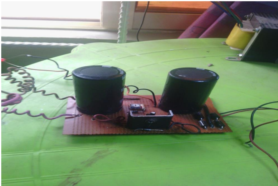
Figure 6: Diode, Heat sink and Capacitor to a vera board
