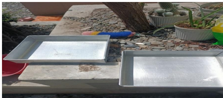
Figure 8. Drying the first layer of the epoxy resin
