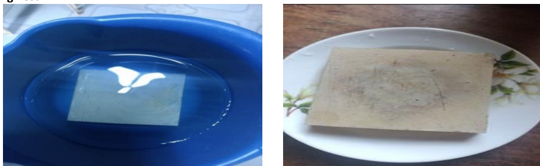
Figure 21. Soaking the fiber decorative tiles surface test.
