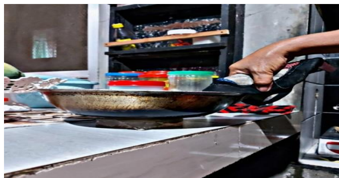
Figure 20. Placing hot frying pan on the tiles surface test.
