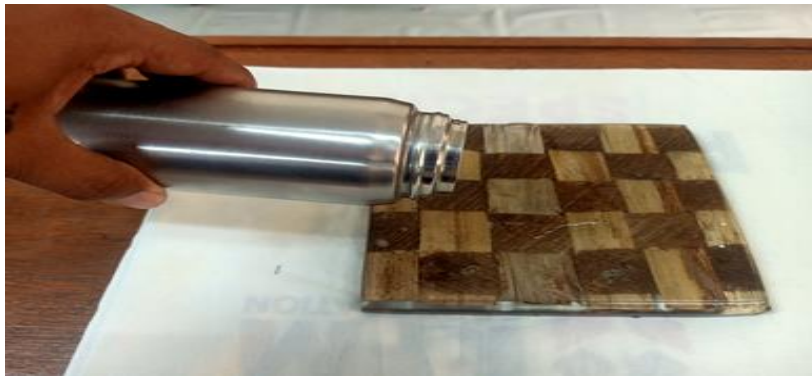
Figure 18. Pouring hot water on develop decorative resin wall tiles with various natural fibers.
