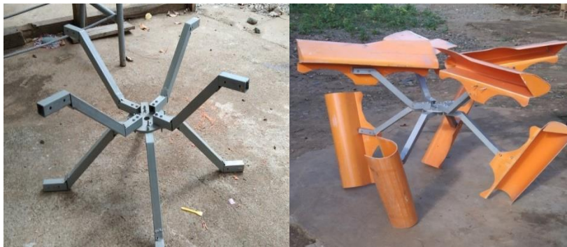
Figure 10. shows the assembled spindle and the Vertical Axis Wind Turbine
