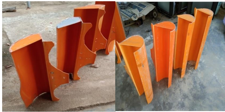
Figure 9. Constructed air foils of the turbine
