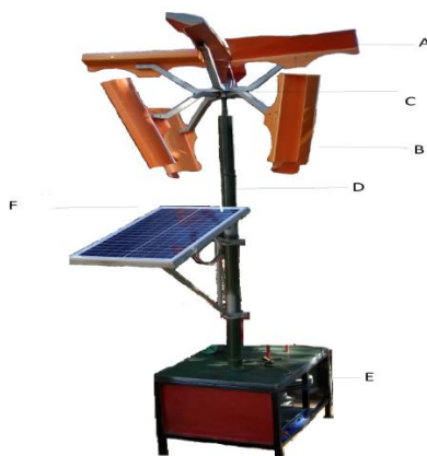
Figure 4. Parts of the Vertical Axis Wind Turbine
