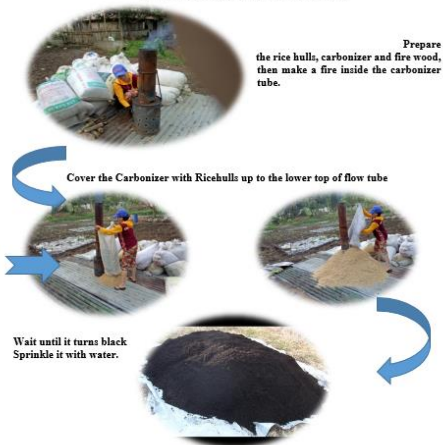
Fig. 1. Procedure in Making Carbonized Rice hulls
