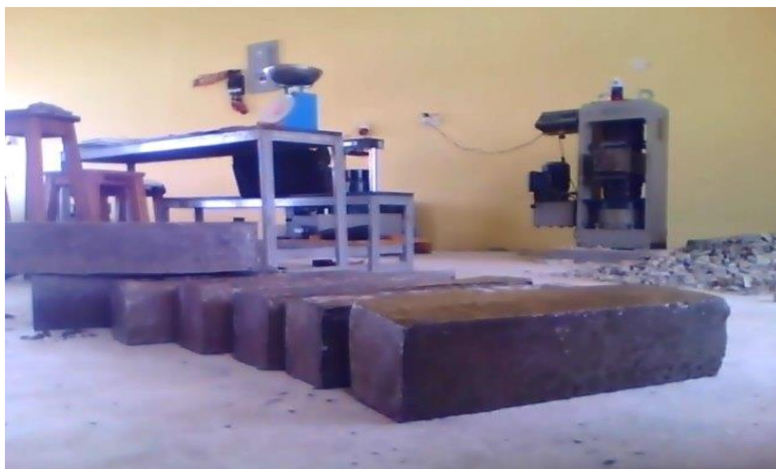
Fig. 1. Flexural Specimen Samples
