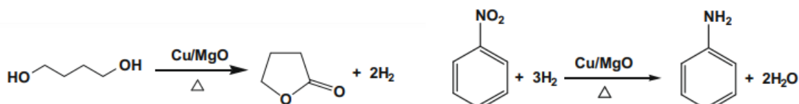
Scheme 1. Catalytic dehydrogenation of 1,4-butanediol to \gamma -butyrolactone.
