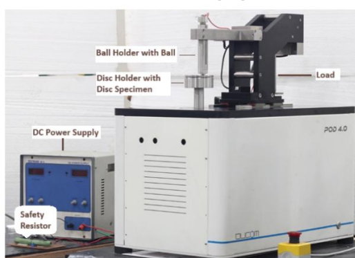
Fig No 1: Electrified Ball on Disc Setup
