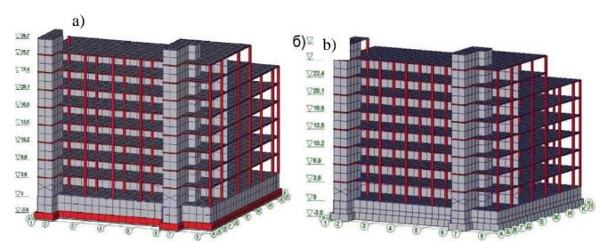
Figure 5. Calculation models: a) seismically isolated building; b) non-seismic isolated building
