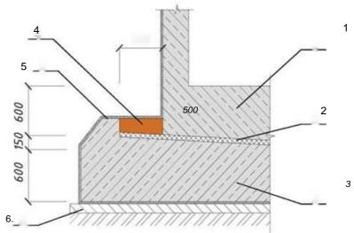
Figure 2. Scheme of a seismic isolation sliding belt:
