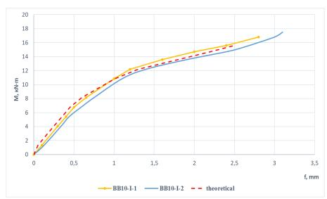
Figure 3. Graph of the dependence of the bending moment on the deflection of the II-series sample beams
