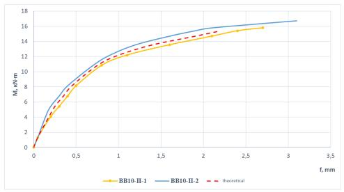
Figure 4. Graph of the dependence of the bending moment on the deflection of the III-series sample beams
