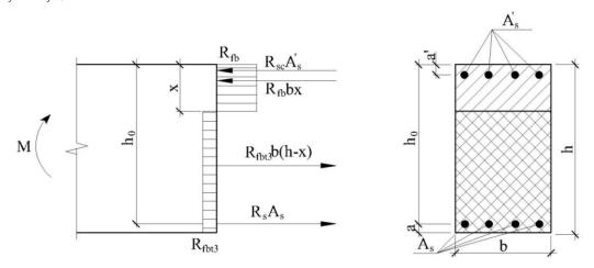
Figure 1. Diagram of forces and stress diagram in a section normal to the longitudinal axis of a bent fiber-reinforced concrete element of rectangular section with reinforcement, when calculating its strength.
