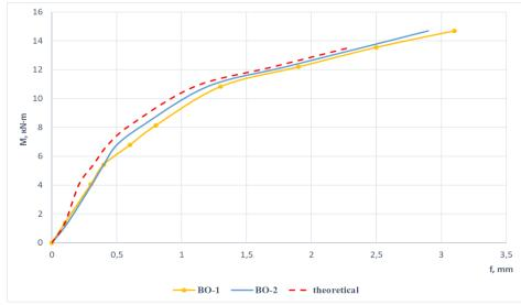
Figure 2. Graph of the dependence of the bending moment on the deflection of the I-series sample beams
